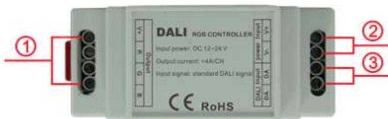
(1) Output: Load output connects with the LEDs need dimming, V+ is positive electrode (voltage is same as supply voltage V+), R, G, B is negative electrode of red, green, blue LED.
