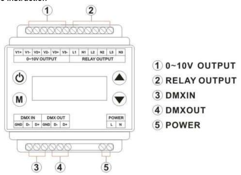
**0-10V OUTPUT**: 3 channel 0-10V dimming signal output interface, each channel maximum current is15mA.
