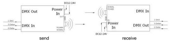
When controller work normally, indicator light SIGNAL will lighten.
