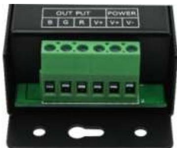
**POWER:** input interface of power, V+ should be connected with positive of power, V- connected with negative of power, the range of supply voltage is DC5-24V
