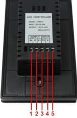
4 and 5: power input, input voltage range: 12-24V, 4 for positive, 5 for negative.
