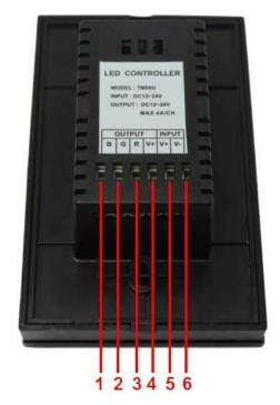
5 and 6: power input, input voltage range: 12-24V, 5 for positive, 6 for negative.
